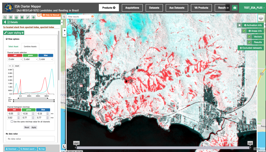
Figure 3 – Illustration of a simple geo-information product generated by retrieving the NDVI variation between two multispectral images in the case of a landslide (Pleiades vs Sentinel-2). Credits: CNES, Airbus, Copernicus, ESA.
