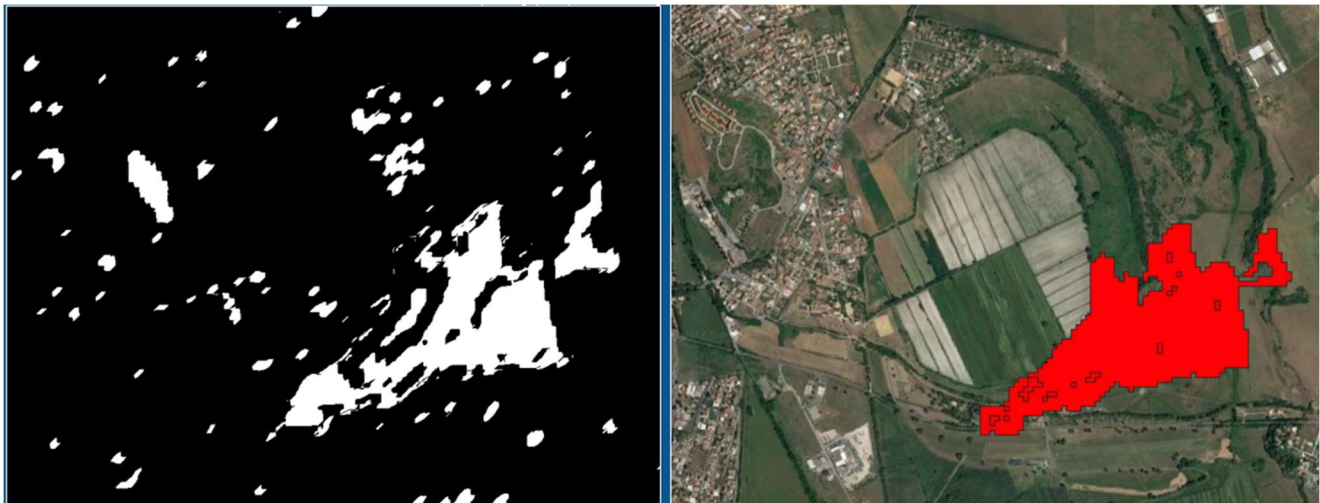
Figure 20. SSIM binarization output (left) and vector of the burnt area generated in QGIS environment (right).
